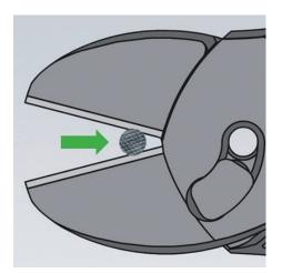
First make a notch in the wire using the KNIPEX TwinForce® until the required hand force increases considerably. Insert the wires as close to the hinge as possible. In case of cutters with very high transmission, the width of the Now open the pliers and slide the wire backwards towards the joint. Hold the cutting edge in the notches you have gap between the cutting edges close to the fulcrum may be less than the thickness of the wire. Wires may slip made in step 1.
