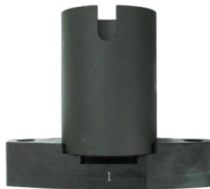
Tool installation for disassembly of silent block
